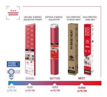
The thermal resistance of a flooring system (floor covering + underlay) should not exceed 0,15 m<sup>2</sup>K/W in accordance with EN 16345 and DIN EN1264.
